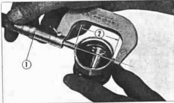
① Micrometer ② Piston diameter Fig. 30
