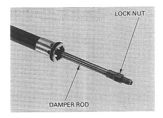
Remove the rebound spring and piston rod from the fork damper.
