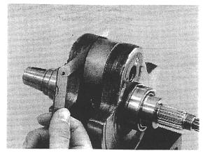
Measure the connecting rod big end radial clearance.
