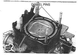
Be careful not to damage the mating surfaces when install the cylinder head.
