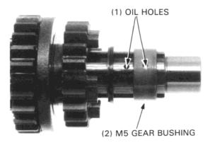
Install the mainshaft and countershaft into the left crankcase together.
