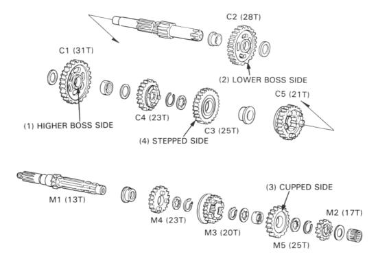
Align the hole in the M5 gear bushing with the hole in the main-shaft when installing.
