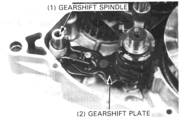
Bend down the lock washer tabs and remove the bolt and lock washer from the center shift fork.
