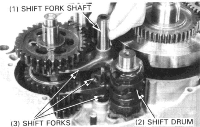
Remove the mainshaft and countershaft as an assembly.
