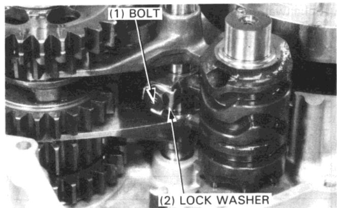
Remove the shift fork shaft, shift drum, and shaft forks.
