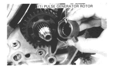
Remove the pulse generator and primary drive gear.
