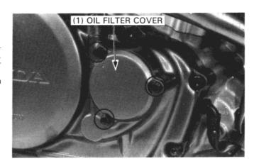
Check that the O-ring on the oil filter cover is in good condition.
