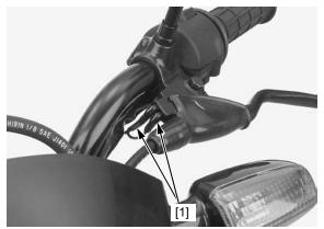
There should be continuity with the clutch lever [1] applied, and there should be no continuity when the clutch lever is released.
