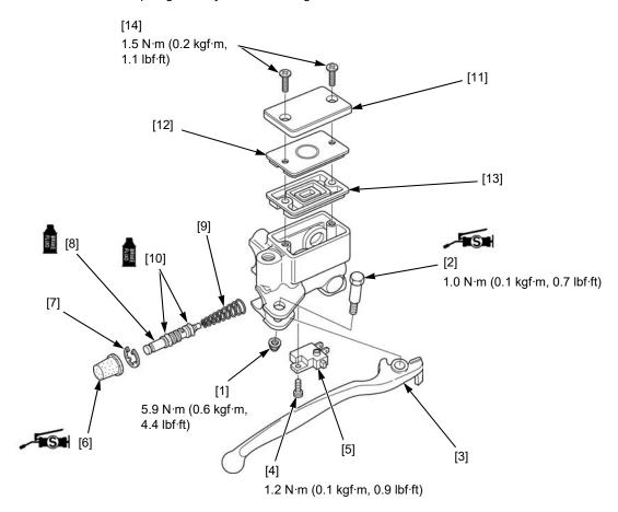
Remove and install the snap ring [1] using the special tool.
