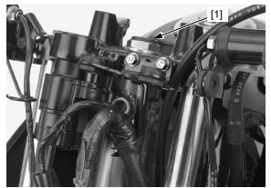
Install the turn signal lights [1] and top bridge pinch bolts [2].
