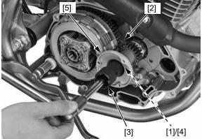
Loosen the clutch lifter plate bolts [1] in a crisscross pattern in several steps.
