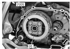
Attach the clutch center holder [1] to the pressure plate using the four clutch lifter plate bolts to hold the clutch center, and then loosen the lock nut [2].
