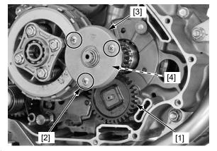
Install the gear holder between the primary drive and driven gears, and loosen the oil filter rotor lock nut [1].
