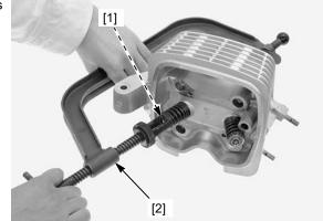
Support the cylinder head above the work bench surface to prevent valve damage.
