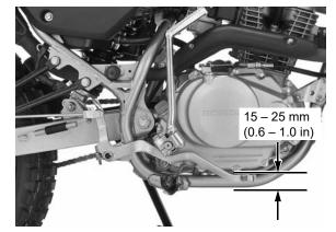
Adjust the freeplay by turning the adjusting nut [1].
