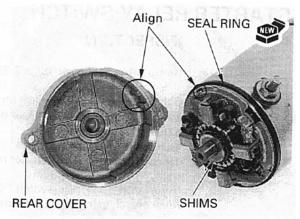
Install and tighten the motor case bolts.
