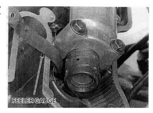
Rotate the crankshaft counterclockwise 270° and align the "R T" mark with index mark. Check the rear cylinder valve clearances.
