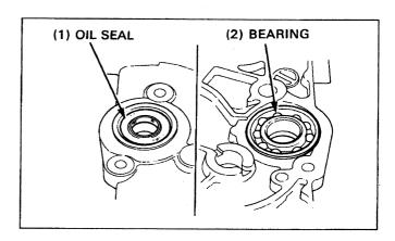
Drive a new bearing into the transmission cover with the marking facing out.
