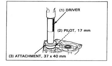
Pull the driveshaft into the bearing in the transmission cover.
