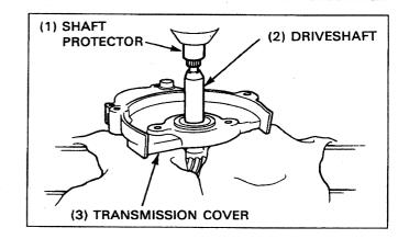
Remove the driveshaft oil seal and bearing from the transmission cover.
