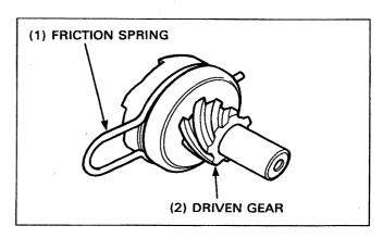
Check the spindle and driven gear bearings for wear or damage.
