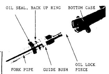
Install fork pipe into bottom case
