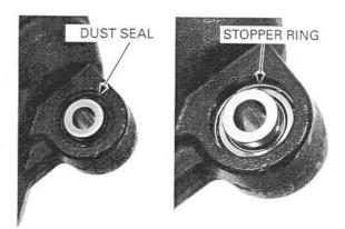
Prepare the following items for the spherical bearing removal.
