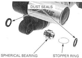
Press a new spherical bearing into the upper mount from the left side using the suitable collar and special tool.
