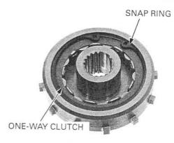
Check the starter clutch outer inner surface and oneway clutch for abnormal wear or damage and replace them if necessary.
