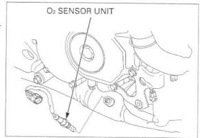
Install the  $O_2$  sensor unit. Tighten the unit to the specified torque.
