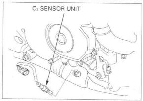
Route the  $O_2$  sensor wire into the frame. Connect the  $O_2$  sensor 4P (Natural) connector.
