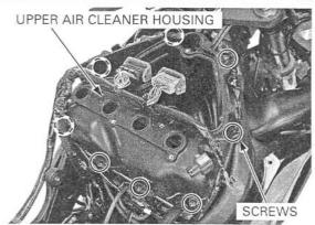
Remove the air funnel/air cleaner housing mounting screws, then remove the air funnels.
