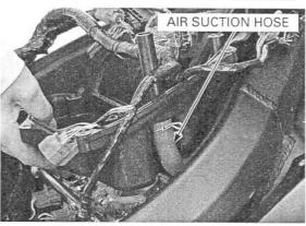
Disconnect the crankcase breather hose from the air cleaner housing.
