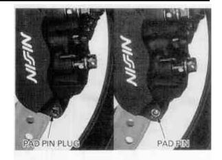
Remove the pad pin and brake pads.
