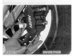
Tighten the pad pin to the specified torque.
