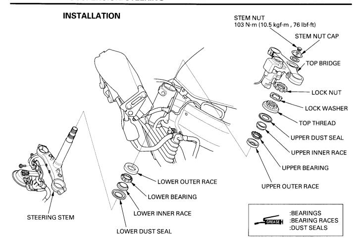
Apply grease to upper and lower bearings and bearing races.
