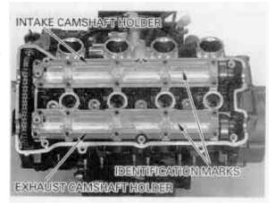
Temporarily install the eighteen holder bolts until the cam holders lightly contact the cylinder head surface.
