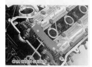
In case the cam sprockets were removed, tighten the cam sprocket bolts to the specified torque.
