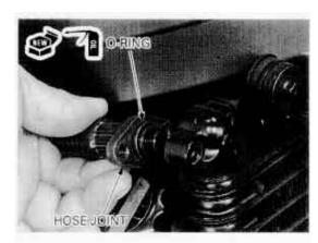
Install the oil hose joints to the oil cooler and tighten the bolts securely.
