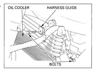
Remove the oil pipe guide mounting bolt.
