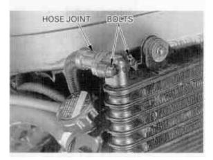
Remove the mounting bolts, main wire harness guide and oil cooler.
