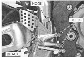
Route the rear brake light switch wire properly. Connect the 2P (Black) connector and secure the brake light switch wire to the wire clamp.
