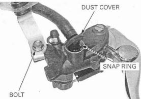
Install the master Install the master cylinder assembly, master cylincylinder holder with der holder and bolts.
