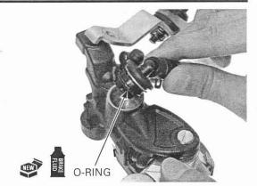
Install the master cylinder reservoir joint into the master cylinder and secure the joint with the snap
