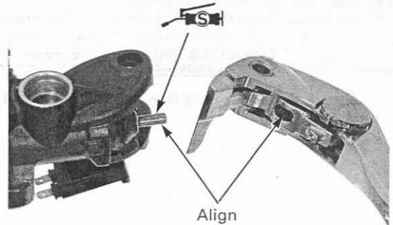
Apply silicone grease to the brake lever pivot bolt sliding surface.
