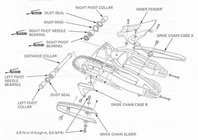
Install the distance collar from the left side pivot. Apply grease (Shell Alvania EP2 or equivalent) to new dust seal lips.
