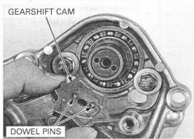
Apply a locking agent to the shift drum cam flange bolt threads. Tighten the bolt securely.
