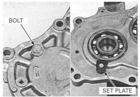
Remove the countershaft bearing using the special tools.
