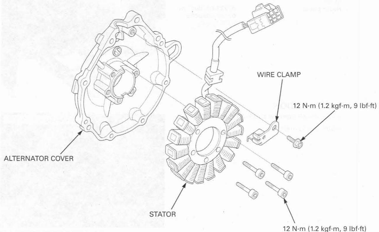
Install the stator into the alternator cover.
