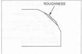
Use a 32-degree cutter to remove the top 1/4 of the existing valve seat material.
