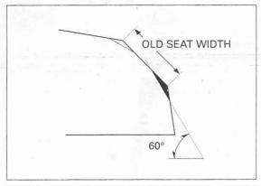
Using a 45-degree seat cutter, cut the seat to the proper width.
