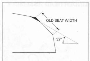
Use a 60-degree cutter to remove the bottom 1/4 of the old seat.
