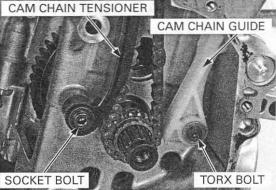
Remove the cam chain and timing sprocket from the crankshaft.
