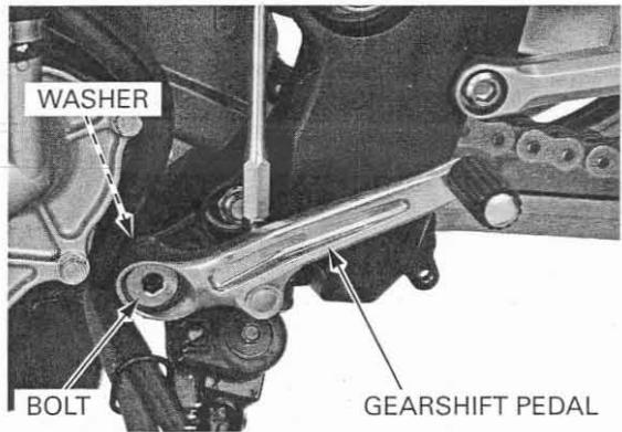
Install the gearshift pedal link to the gearshift spindle while aligning its slit with the punch mark on the gearshift spindle.
