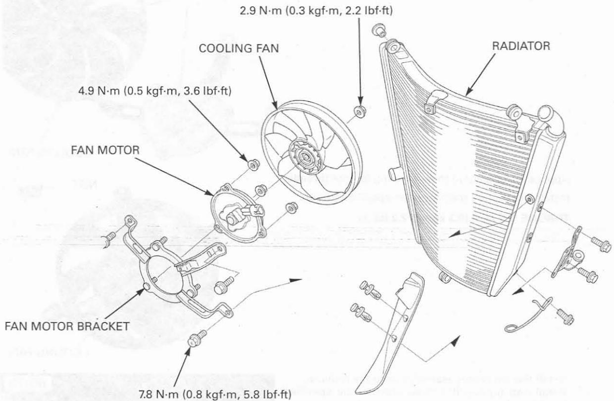
Install the fan motor onto the fan motor bracket and tighten the nuts to the specified torque.
