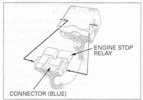
Connect the ohmmeter to the engine stop relay connector terminals.
