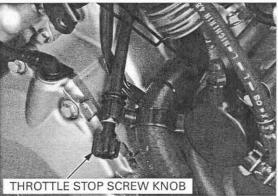
Remove the vacuum gauge from the vacuum hoses. Connect the each vacuum hoses to the 5-way joint. Reset the ECM failure code (page 6-10).
