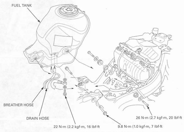
Install the fuel tank, collars and pivot bolts into the frame and tighten the bolts securely.
