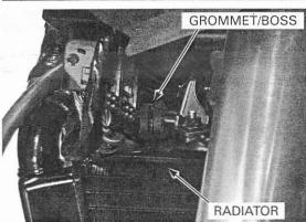
Install and tighten the radiator upper mounting bolt.
