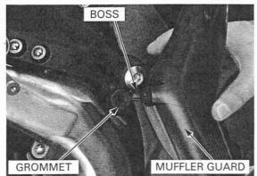
Install the pan screw, collar and screw, then tighten the screws securely.
