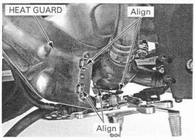
Install and tighten the exhaust pipe heat guard mounting pan screw.
