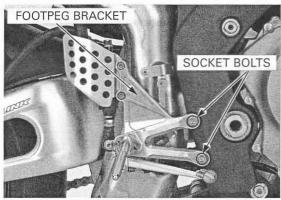
Install the right passenger footpeg bracket onto the seat rail, then tighten the socket bolts to the specified torque.
