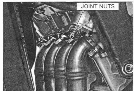
Remove the exhaust pipe mounting bolt/washer, then remove the exhaust pipe.
