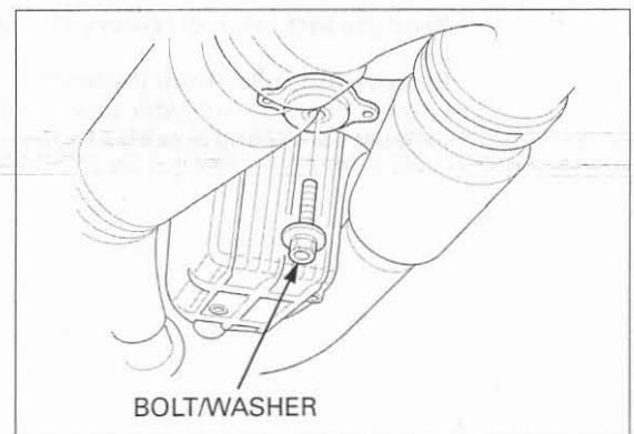
Remove the bolt and exhaust joint pipe clamp.
