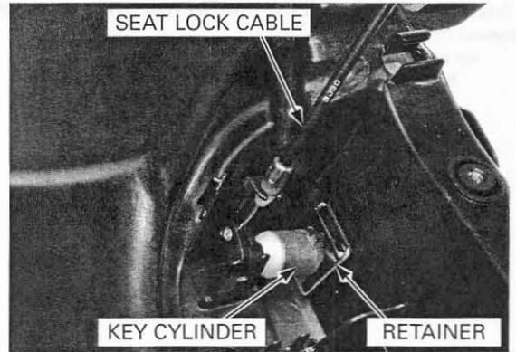
Hook the seat lock cable to the seat lock lever.
