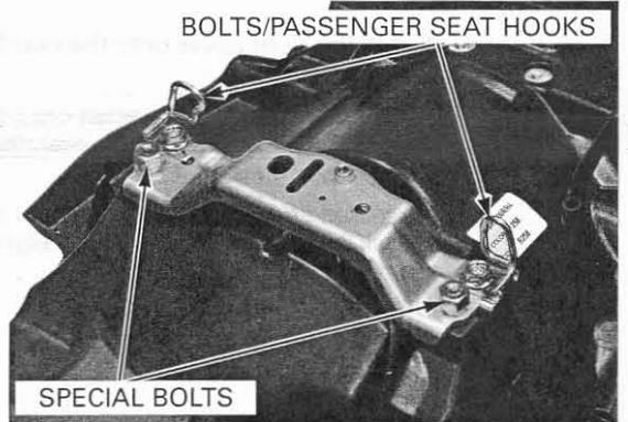
Install the passenger seat rear hook and tighten the pan screw securely.
