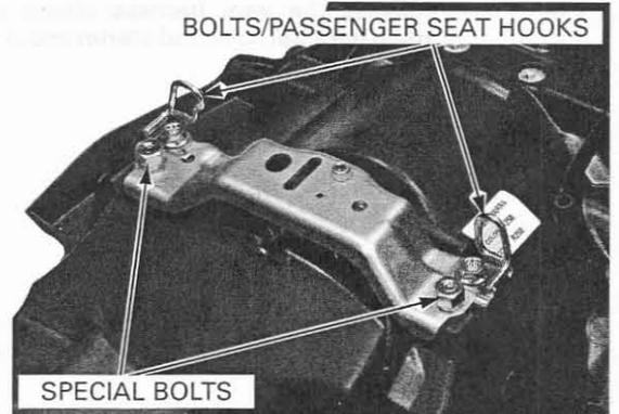
Unhook the seat lock cable from the seat lock lever, then remove the passenger seat bracket.
