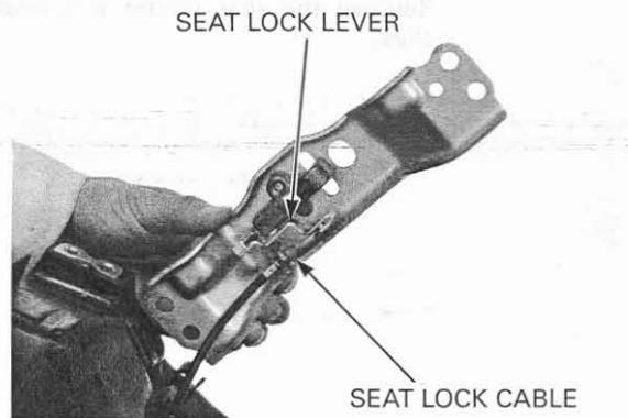
Disconnect the seat lock cable from the seat lock key cylinder. Remove the retainer and remove the seat lock key cylinder from the rear fender B.
