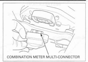
Release the upper cowl off the rearview mirror bolt hole studs and bosses of the upper cowl from the meter stay grommets, then remove the upper cowl assembly.
