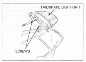
Remove the two screws, trim clip and air duct. Install the air duct and tail/brake light unit in the reverse order of removal.
