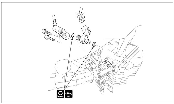
• Quick connect fitting (injector side) →2-2
